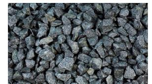
¾" minimum crushed black basalt
