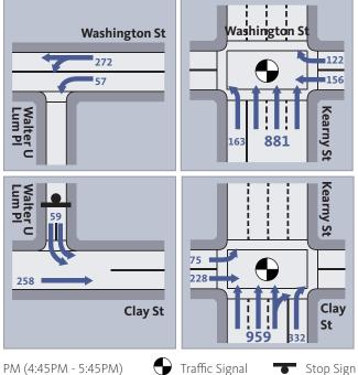
Figure 3.5 Intersection Turning Movements
