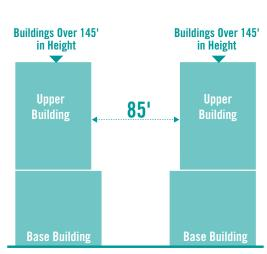
**Figure 6.5.5** Upper Building Separation for Midrise Towers on Different Blocks
