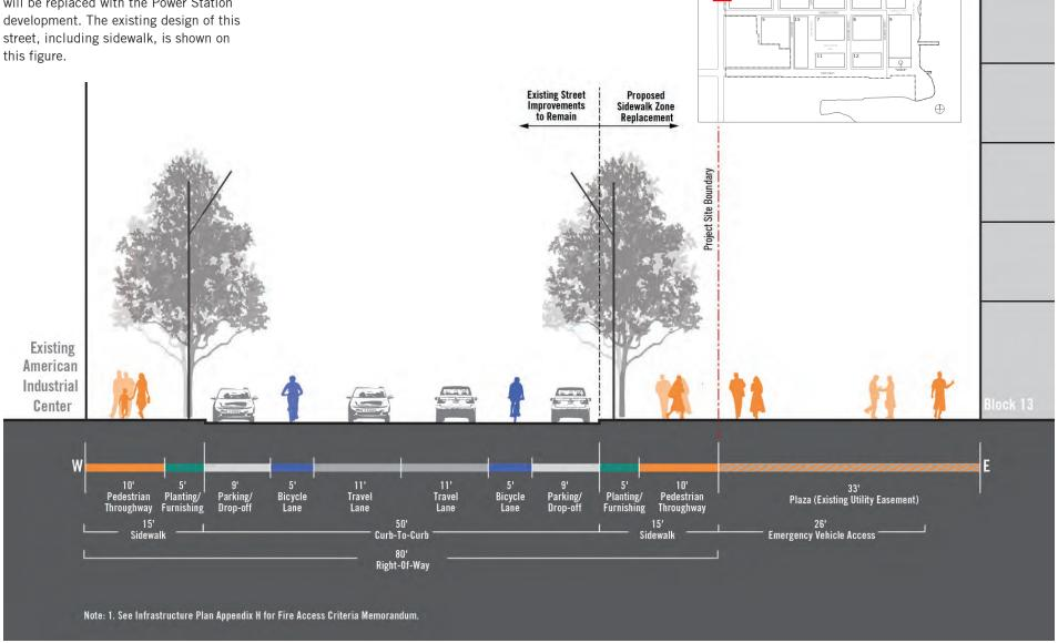
Figure 5.25.1 Illinois St Section - A
