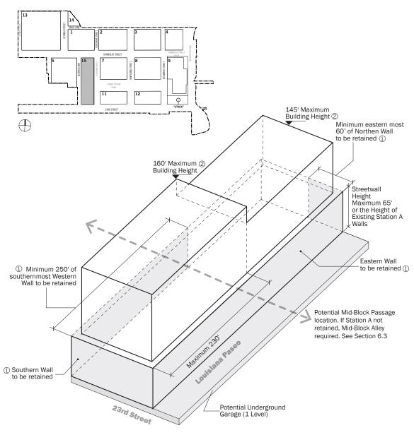
Figure A.6.2 Block 15 Bulk Controls Axon
