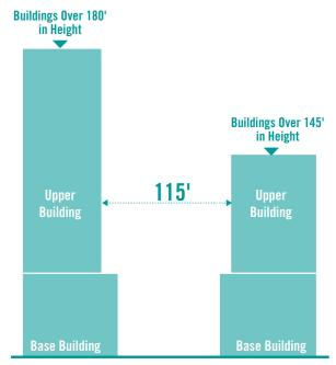
Figure 6.5.6 Upper Building Separation for Midrise and Highrise Towers on Different Blocks
