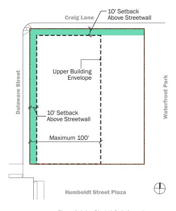
Figure A.4.1 Block 4 Bulk Controls
