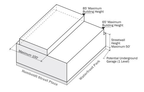
Figure A.4.2 Block 4 Bulk Controls Axon
