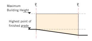
Figure 6.2.2 Measuring Height on a Slope
