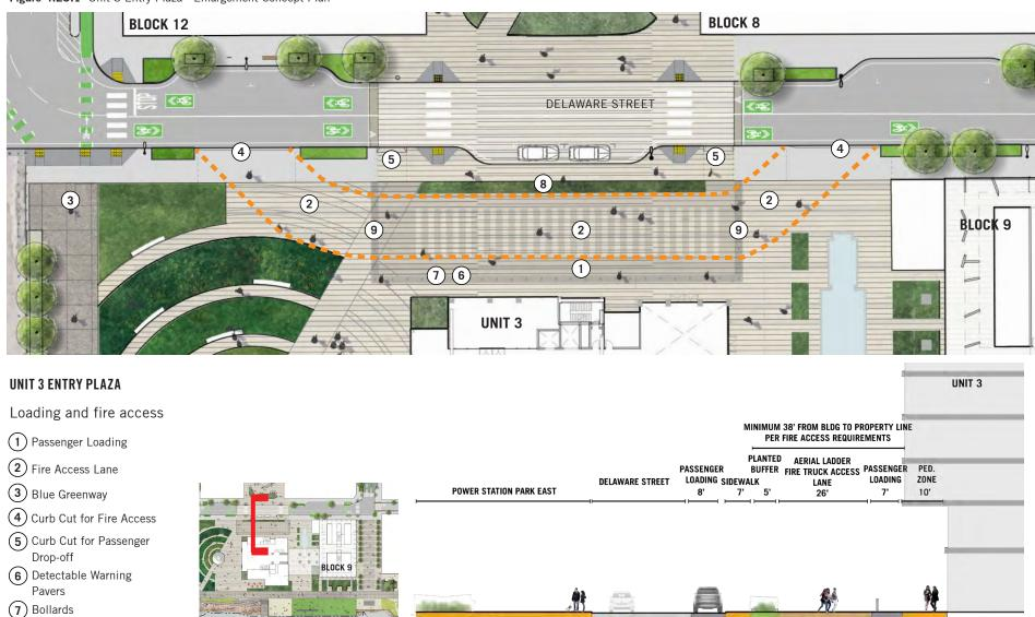
Figure 4.23.2 Unit 3 Passenger Entry Plaza: Concept Section Looking North
