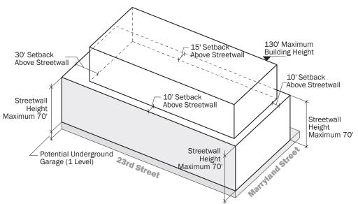
Figure A.10.2 Block 11 Bulk Controls Axon
