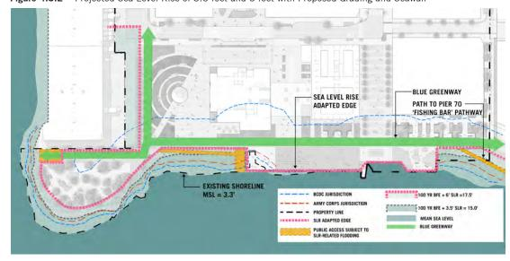
Figure 4.3.2 Projected Sea Level Rise of 3.5 feet and 6 feet with Proposed Grading and Seawall
