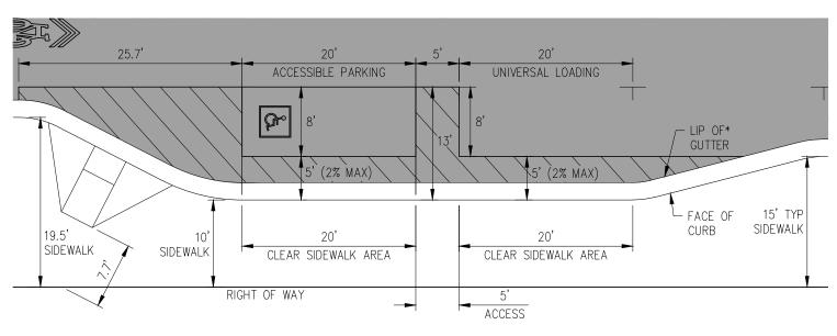
Figure 5.10.2 Universal Passenger Loading Zone and Accessible Parking Stall
