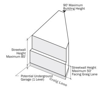
Figure A.13.2 Block 14 Bulk Controls Axon
