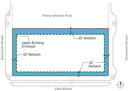
Figure A.11.1 Block 12 Bulk Controls
