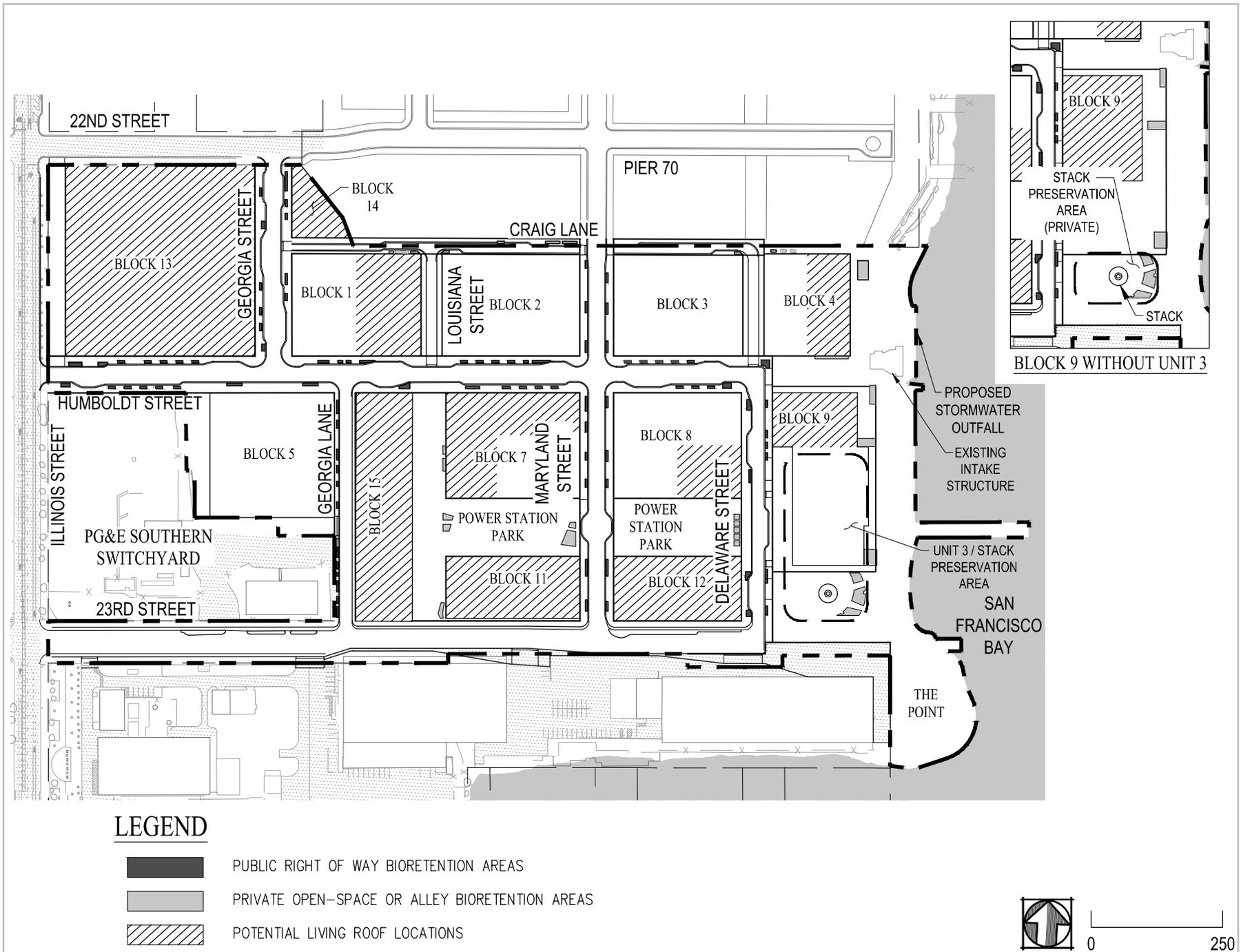
Figure 16.2 Conceptual Stormwater Control Plan
