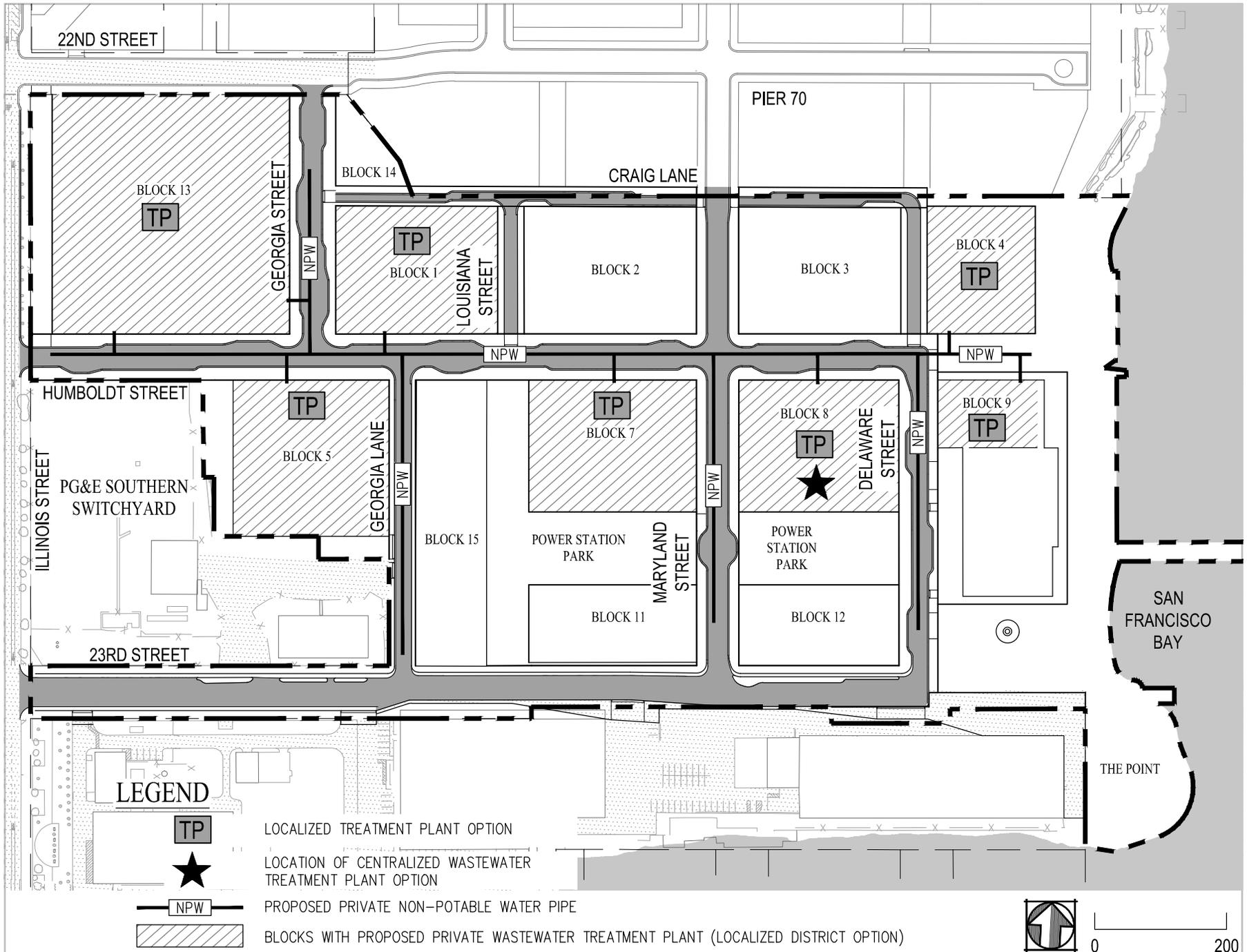
Figure 12.1 Proposed Non-Potable Water System - Localized District and Centralized District Treatment Plant Options
