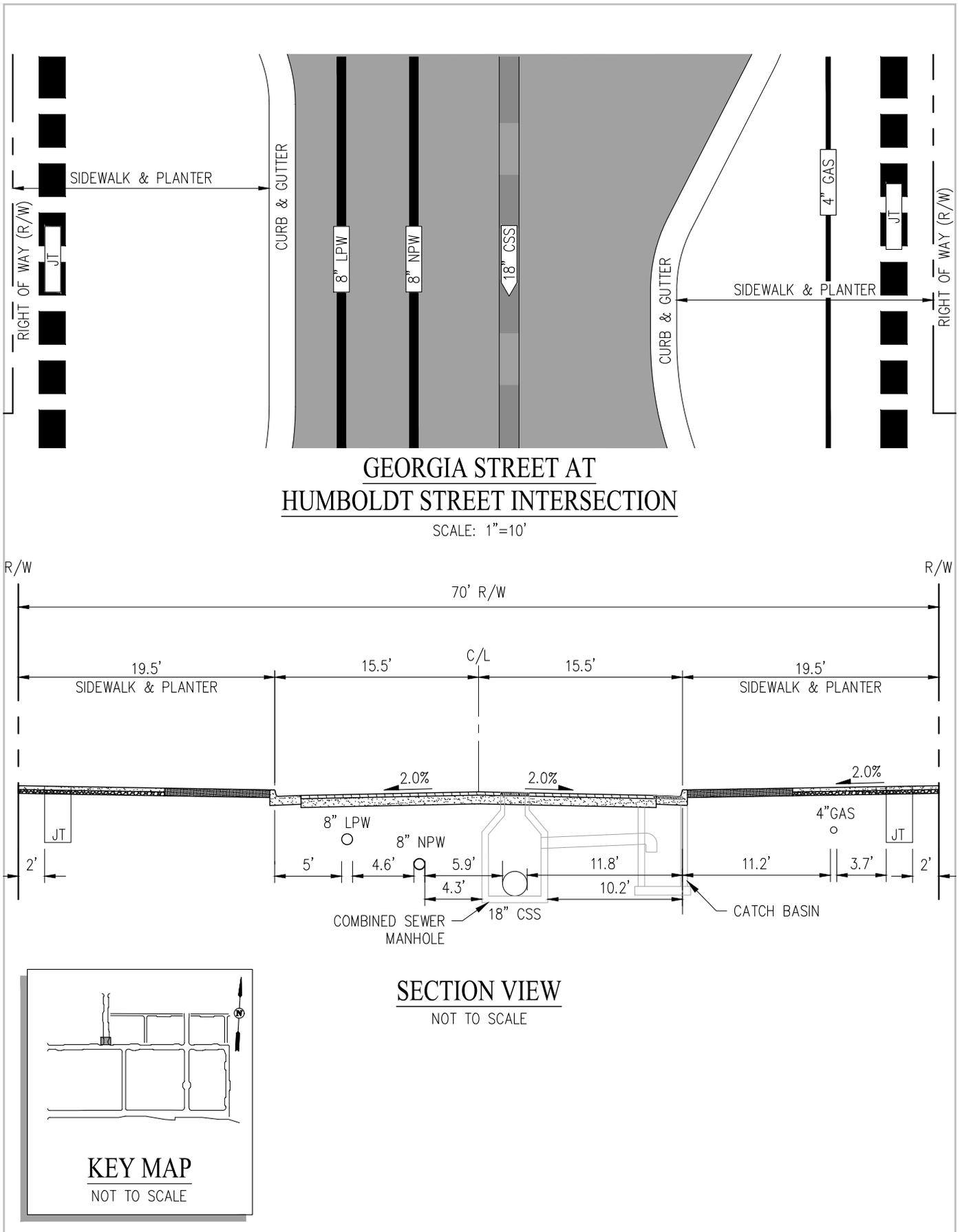
**Figure 10.2 Utility Configurations**
