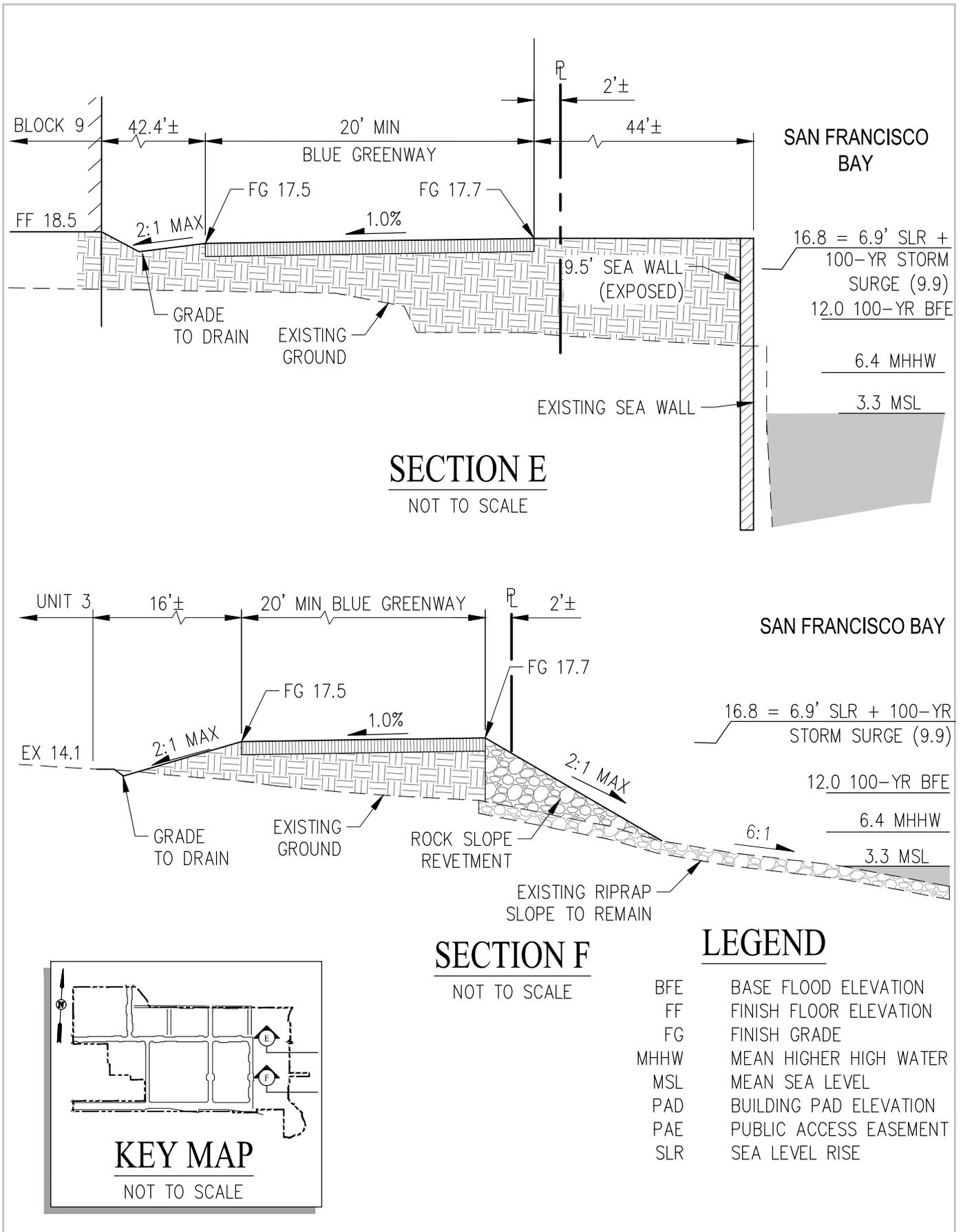
Figure 7.5 Grading Cross Sections at Project Boundaries - Section E & F
