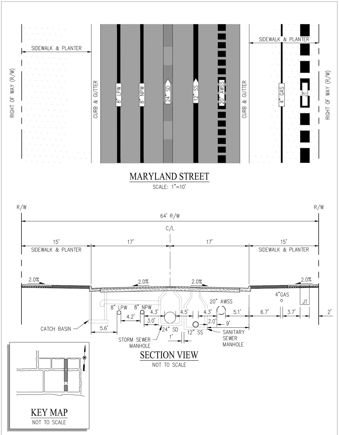
Figure 10.2 Utility Configurations
