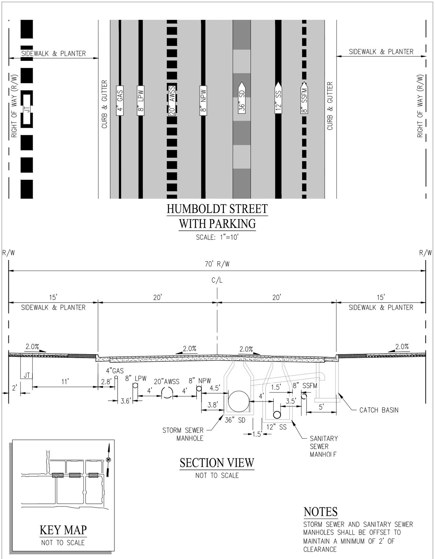
Figure 18.4 Alternative Utility Configurations
