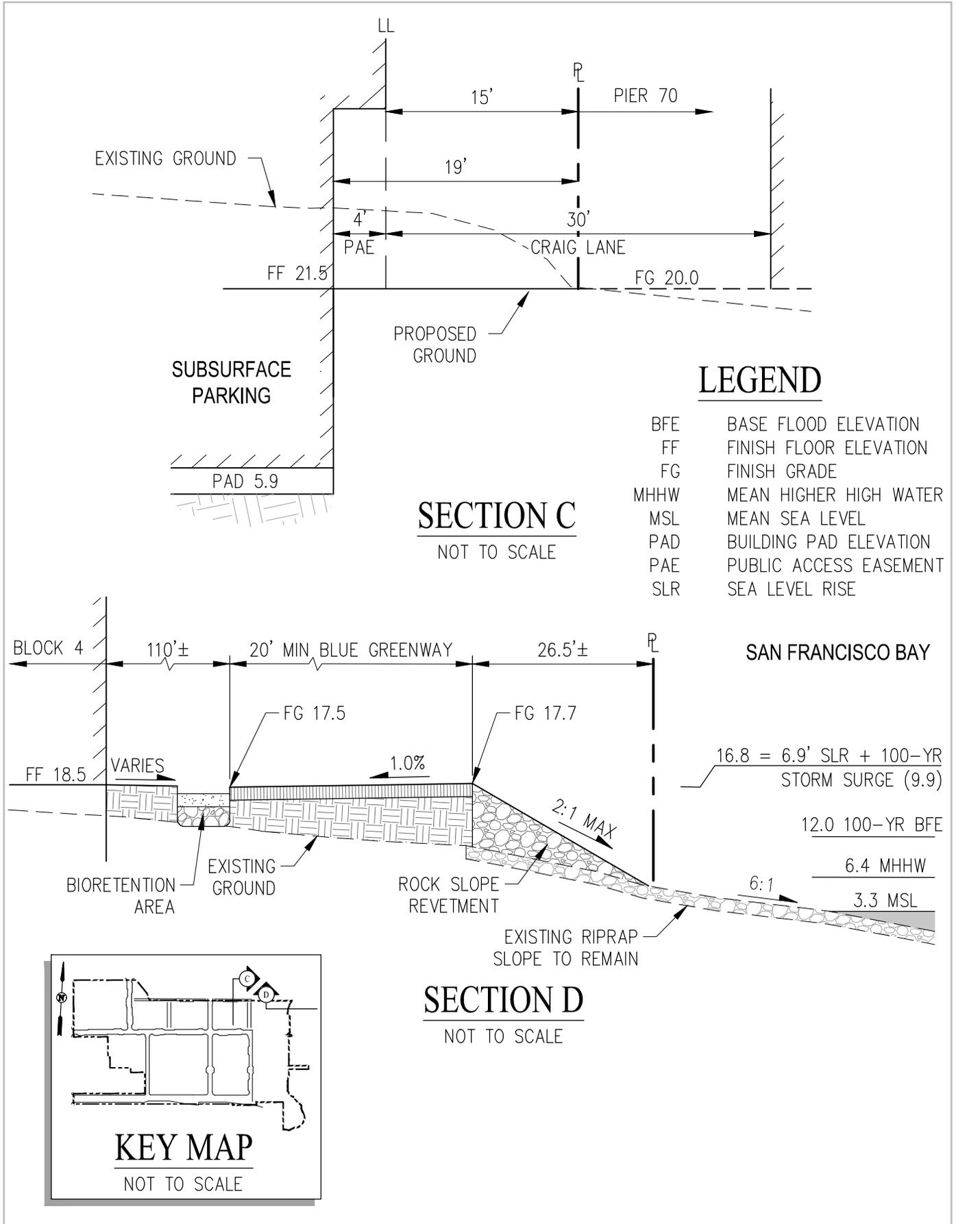
Figure 7.5 Grading Cross Sections at Project Boundaries - Section C & D
