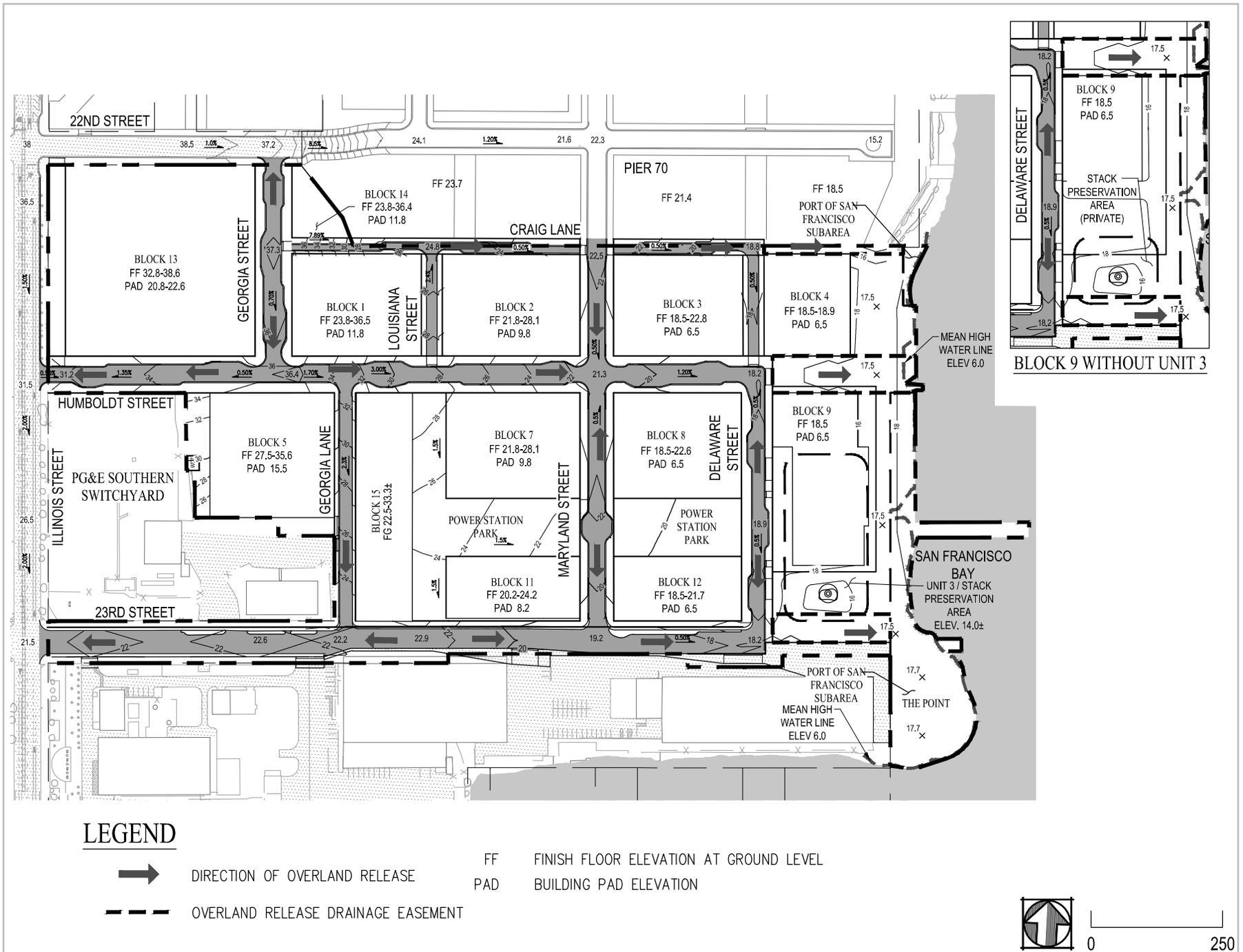
Figure 7.2 Proposed Site Grading
