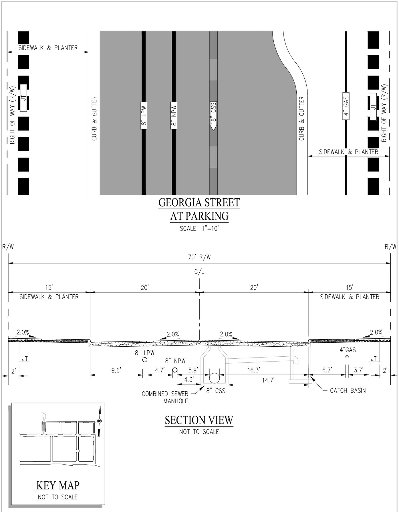
Figure 10.2 Utility Configurations
