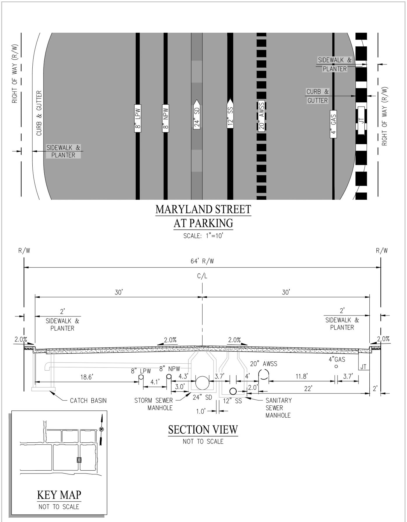
Figure 10.2 Utility Configurations
