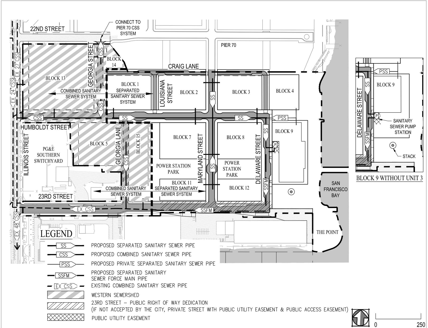
**Figure 14.3 Proposed Combined and Separated Sanitary Sewer Systems**
