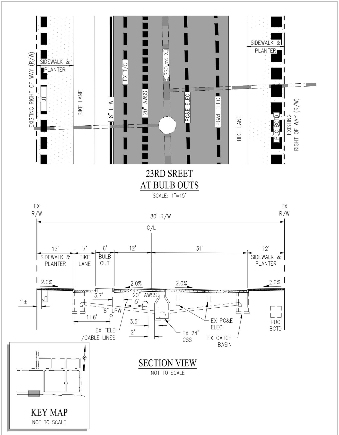
Figure 10.2 Utility Configurations
