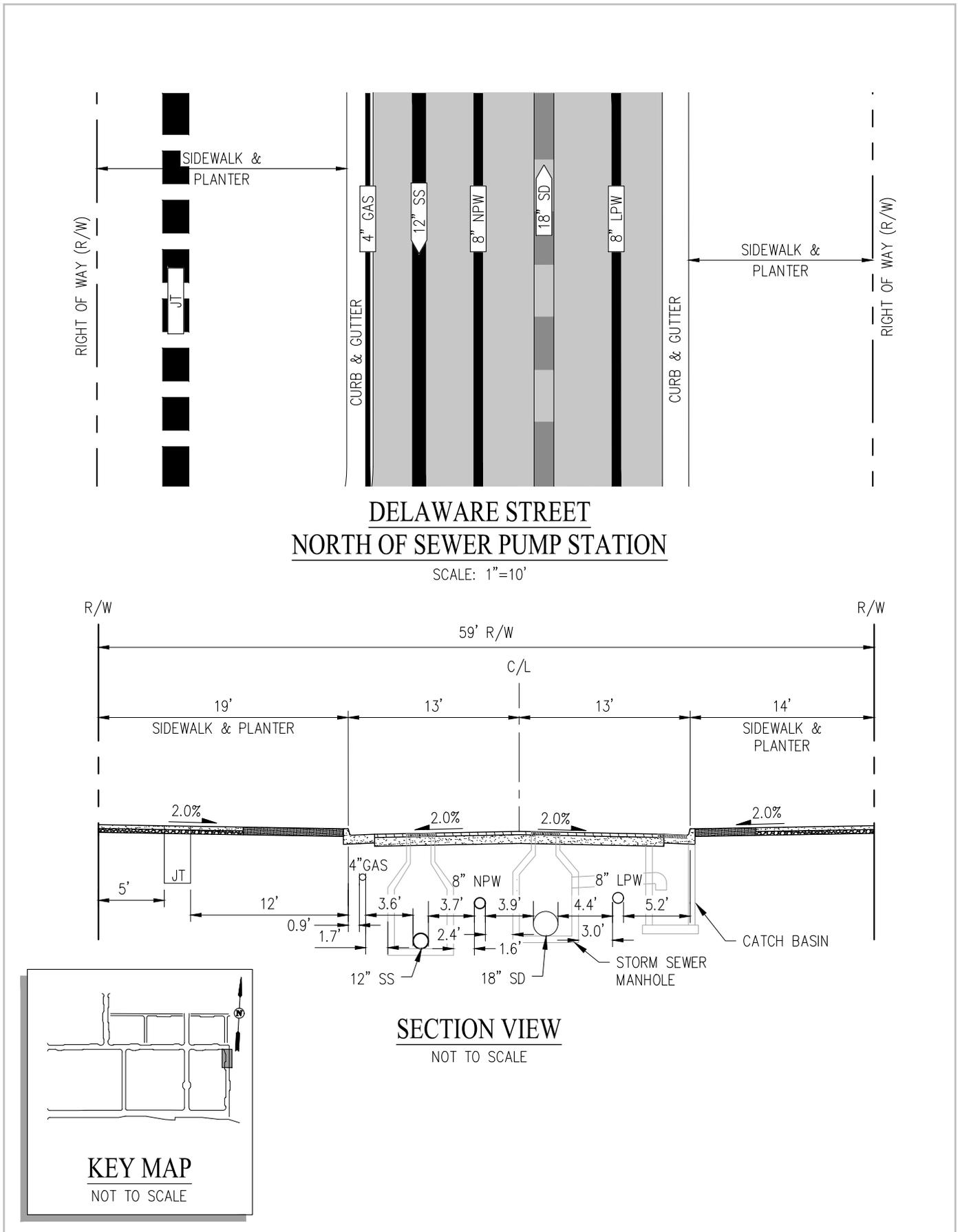
**Figure 10.2 Utility Configurations**
