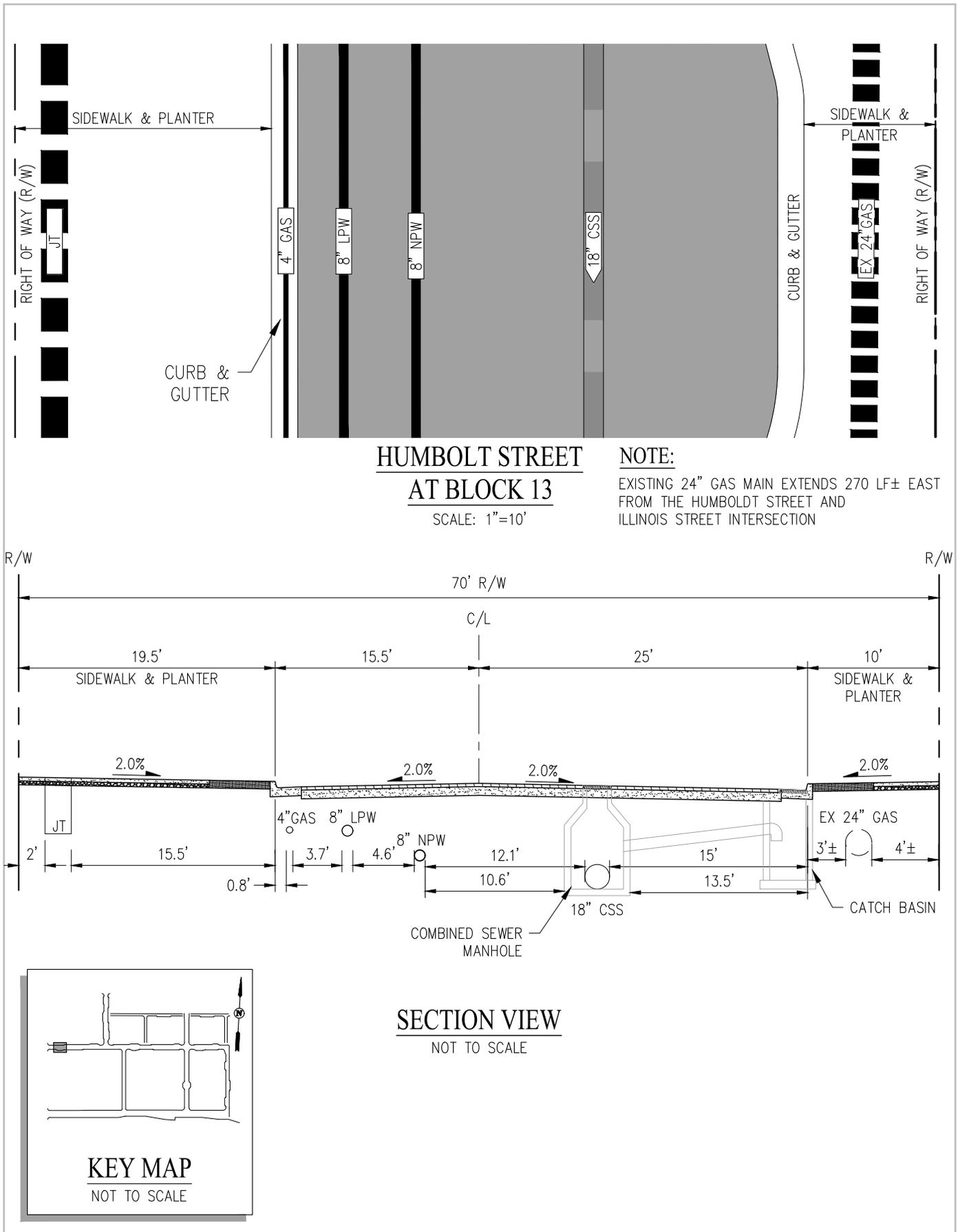
Figure 10.2 Utility Configurations
