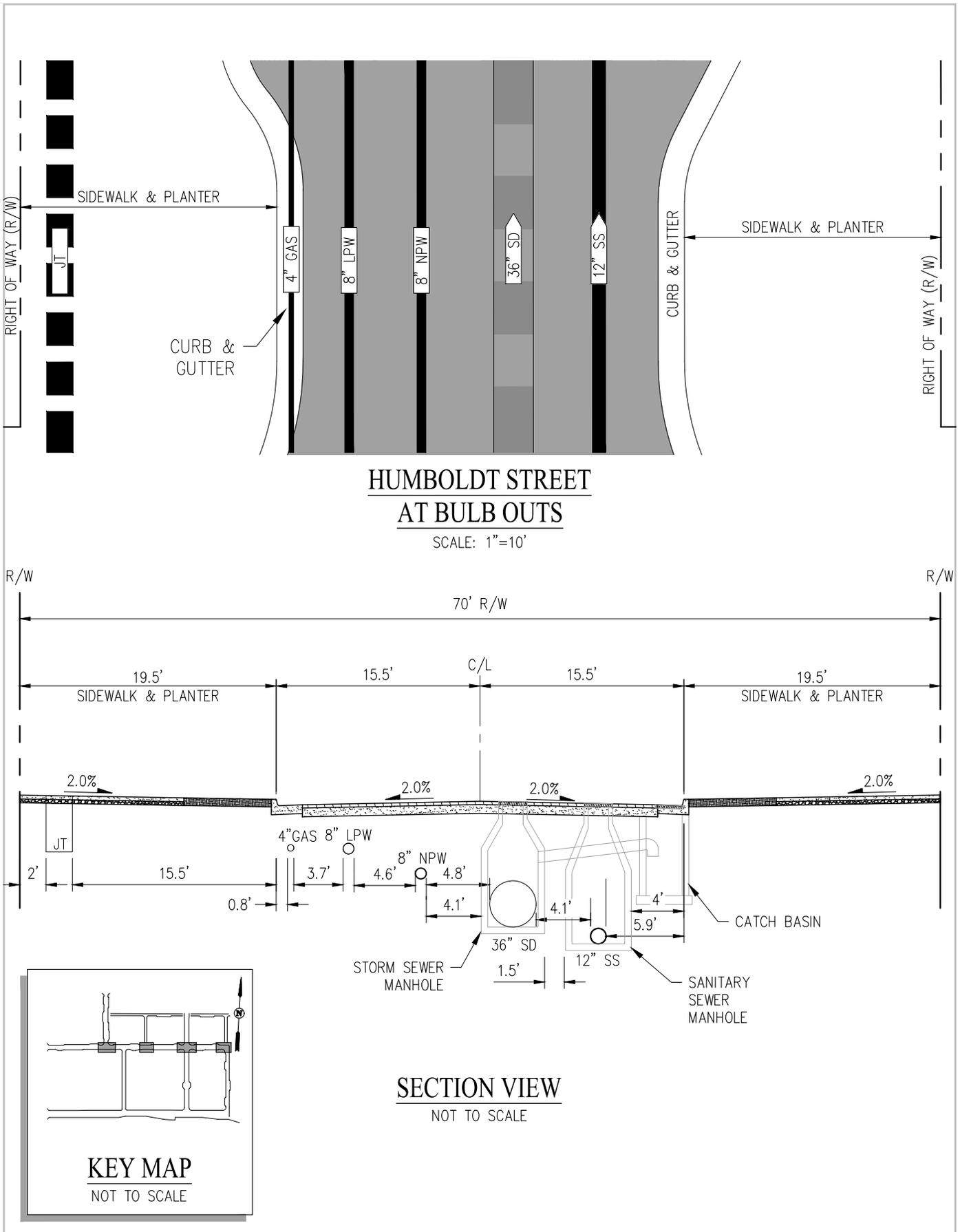
Figure 10.2 Utility Configurations
