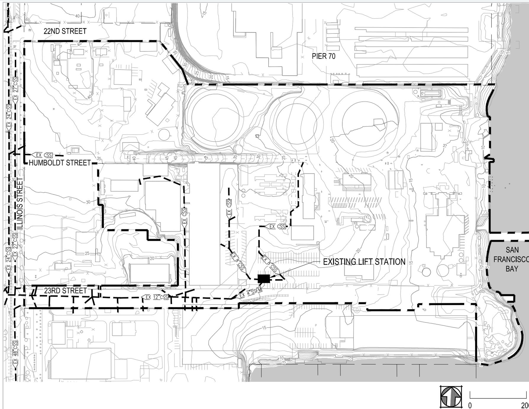
Figure 14.1 Existing Combined Sewer System
