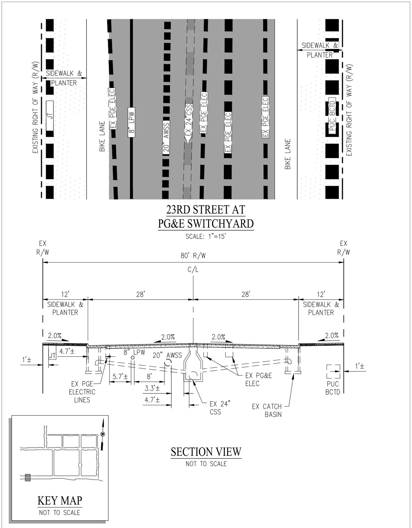
**Figure 10.2 Utility Configurations**
