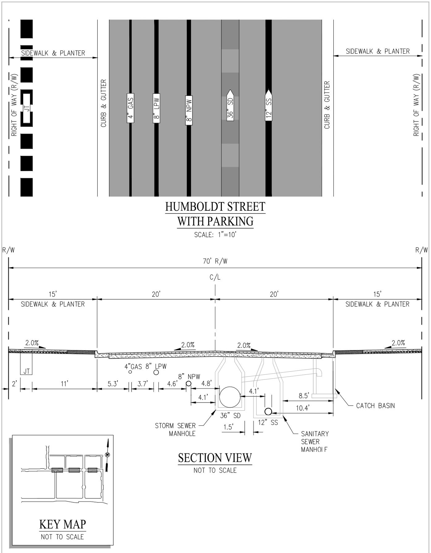
Figure 10.2 Utility Configurations
