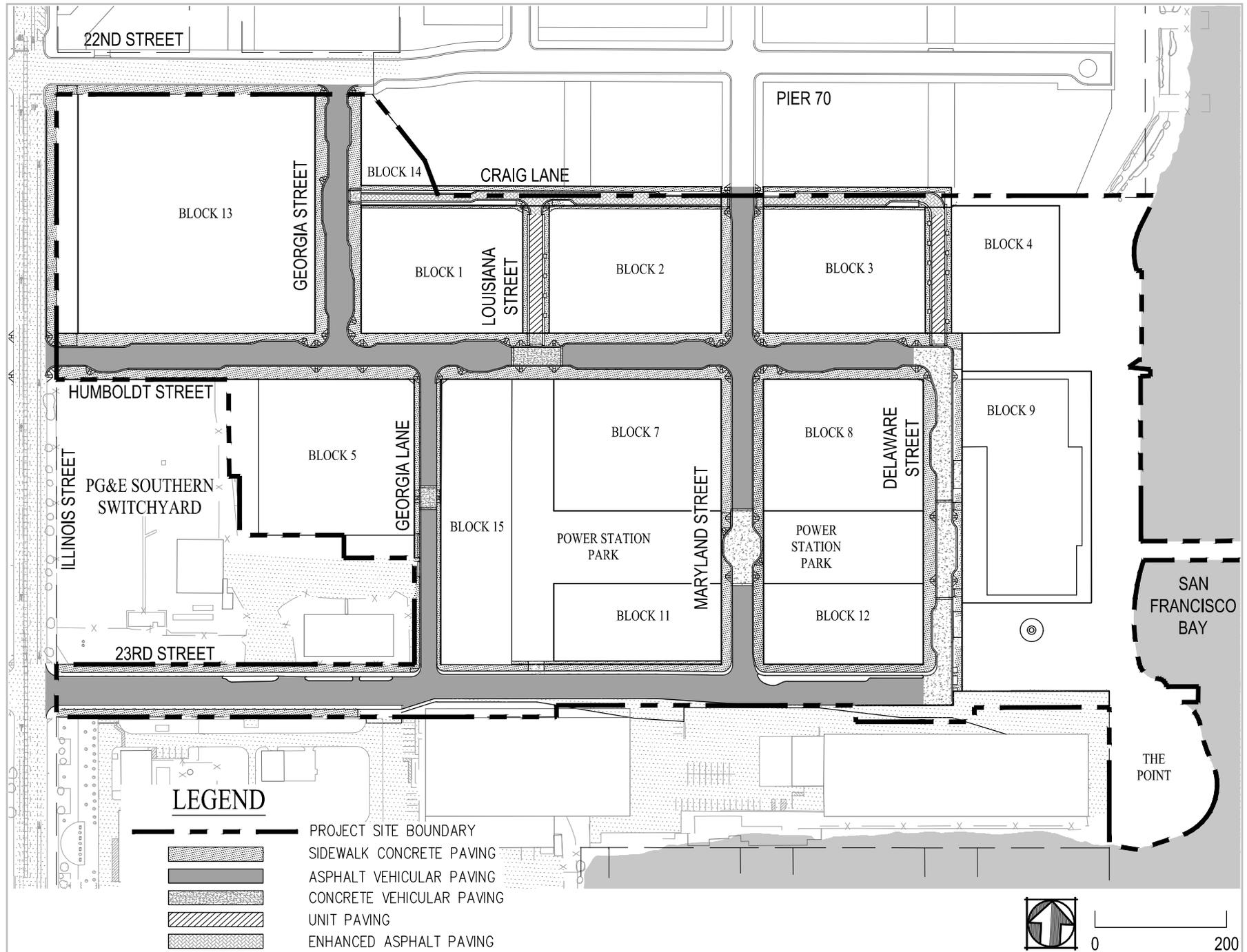
Figure 8.10 Pavement Surfaces
