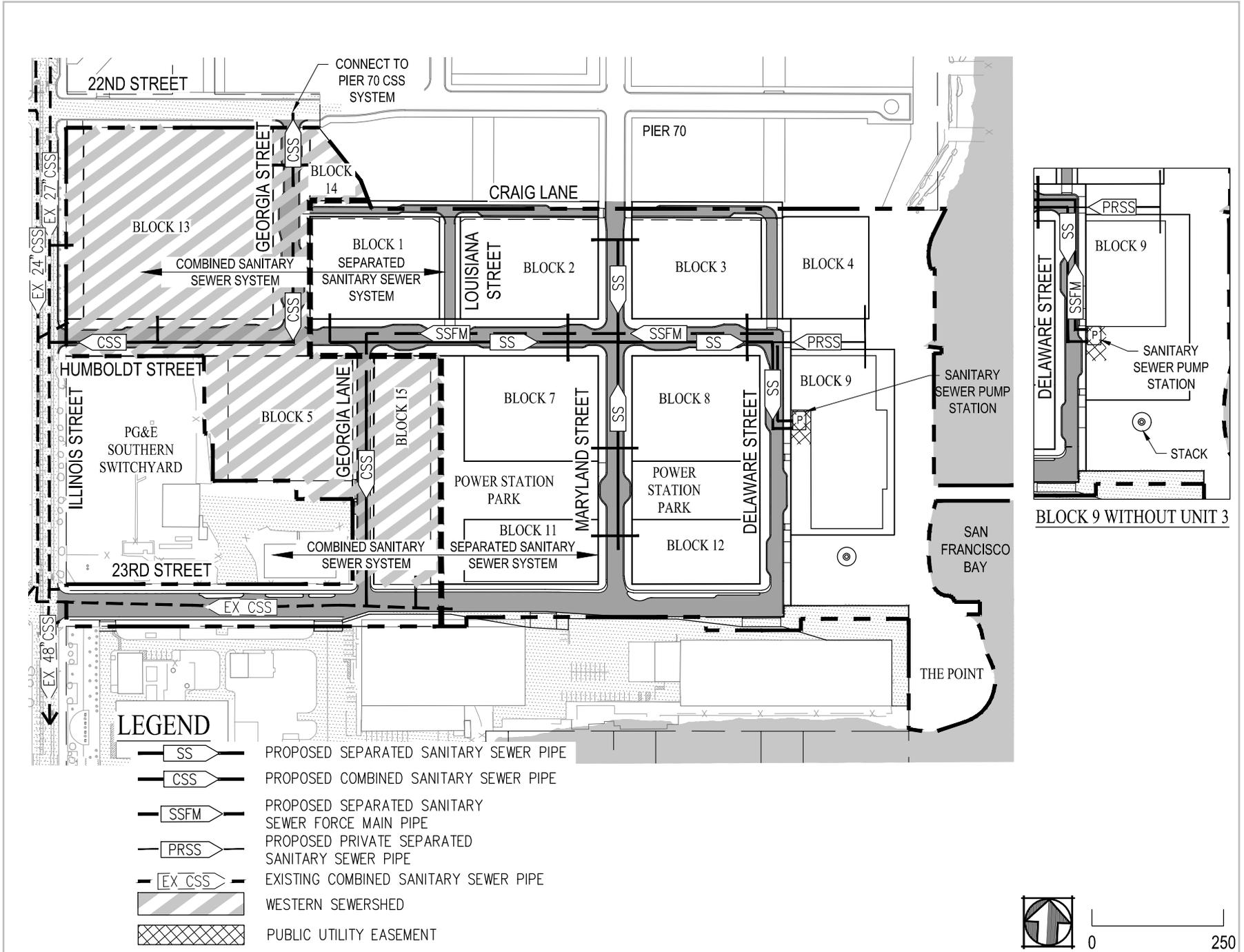
Figure 18.2 Proposed Alternative Combined and Separated Sanitary Sewer Systems
