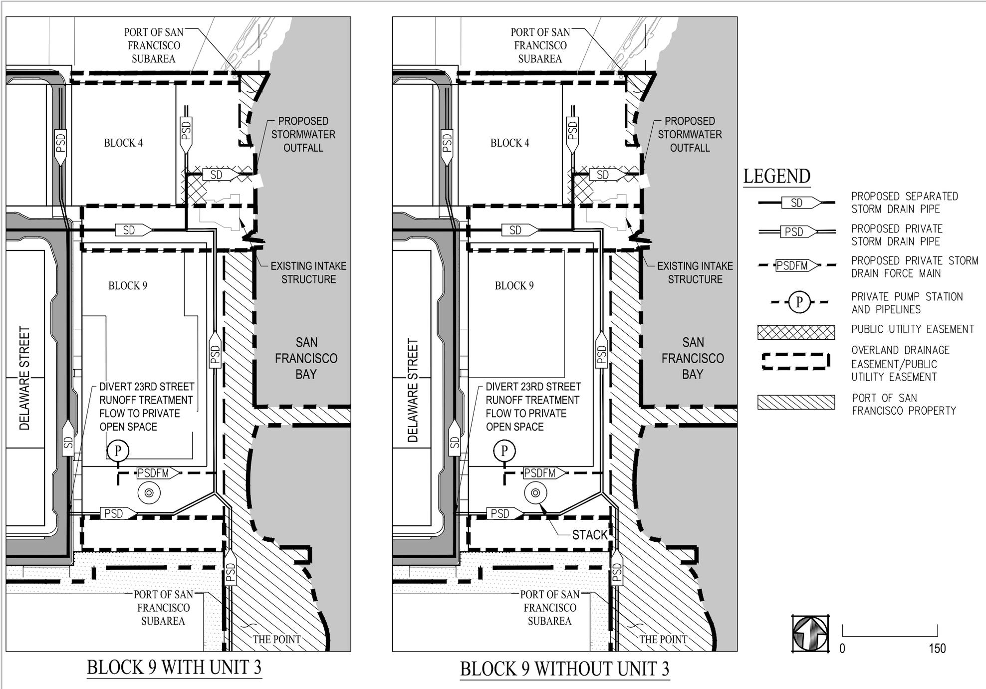
**Figure 15.3 Proposed Storm Drain Systems**
