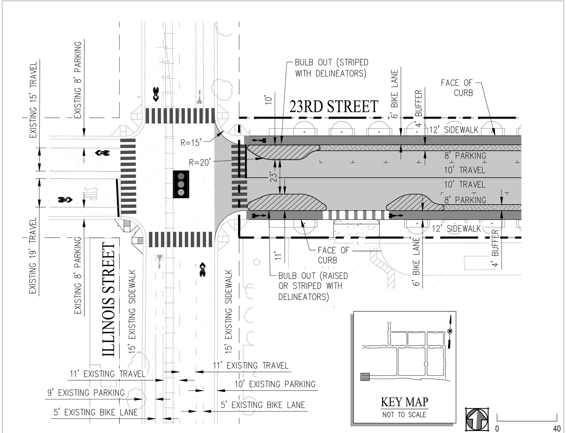
Figure 8.8 Intersection Geometry (Illinois Street & 23rd Street)
