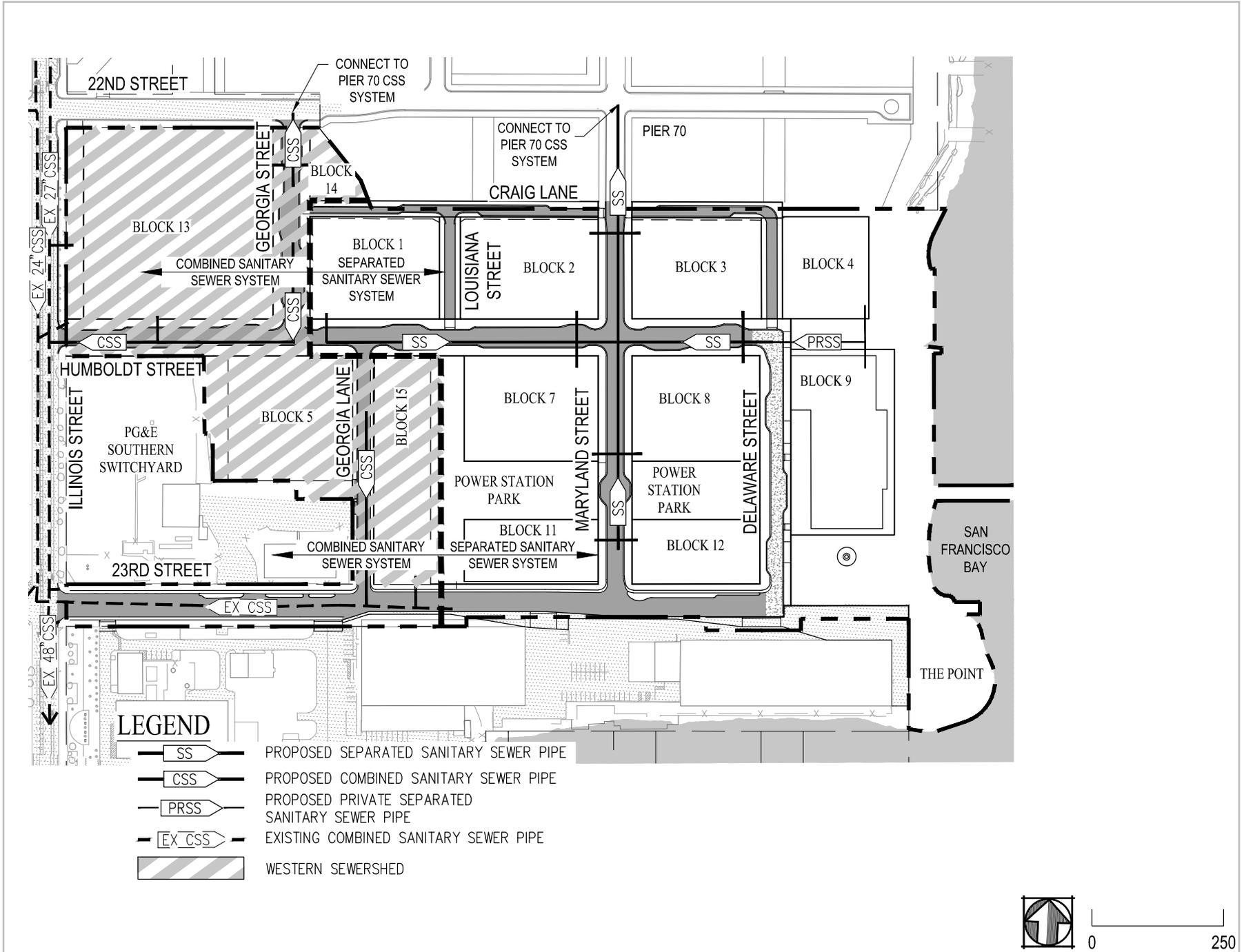
Figure 18.3 Proposed Separated Sanitary Sewer - Northern Connection Alternative
