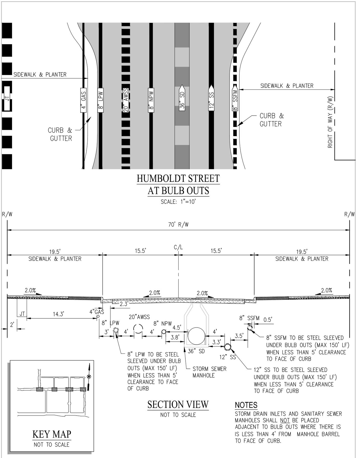
Figure 18.4 Alternative Utility Configurations
