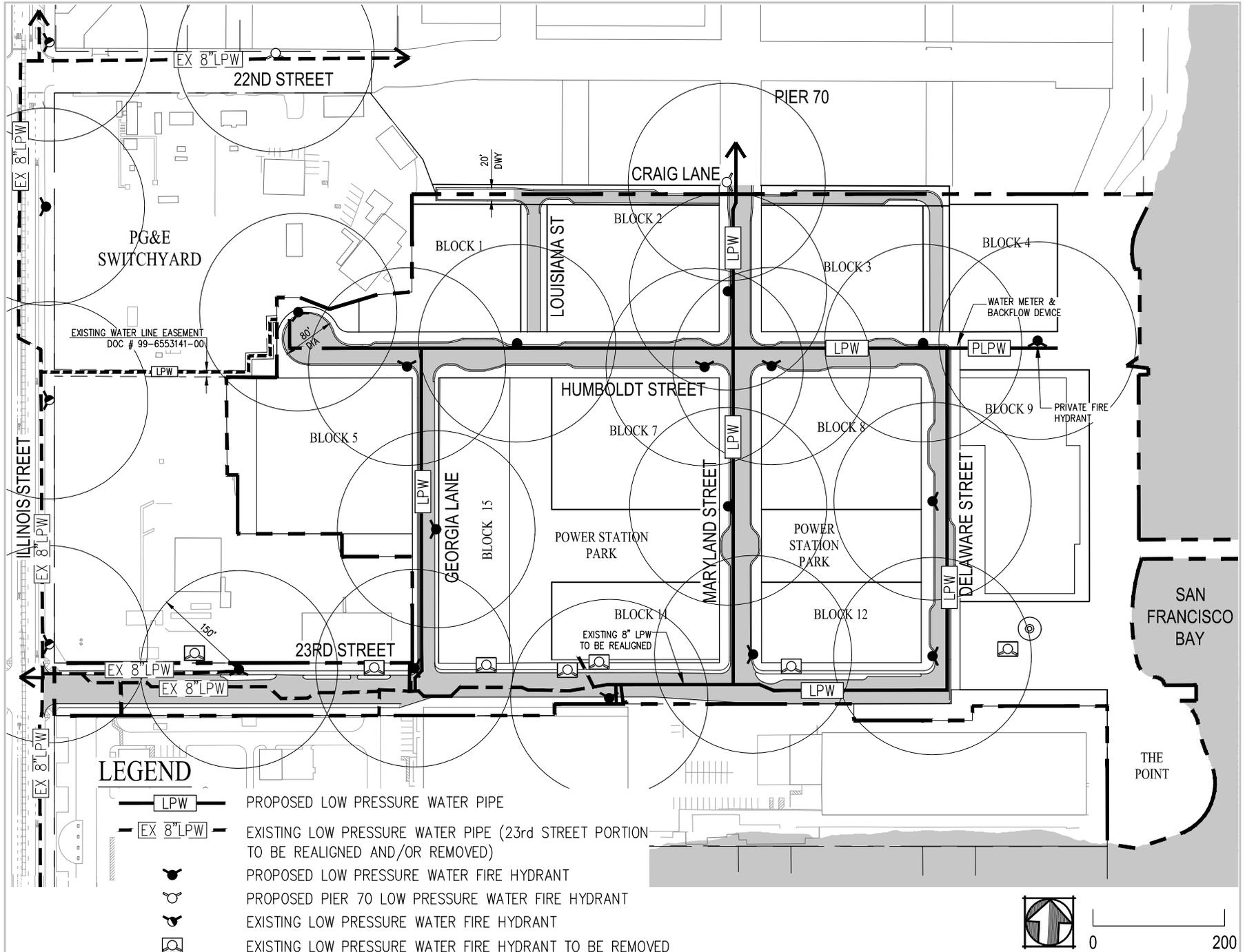
Figure 19.2 No PG&E Subarea Scenario – Proposed Fire Hydrant Locations
