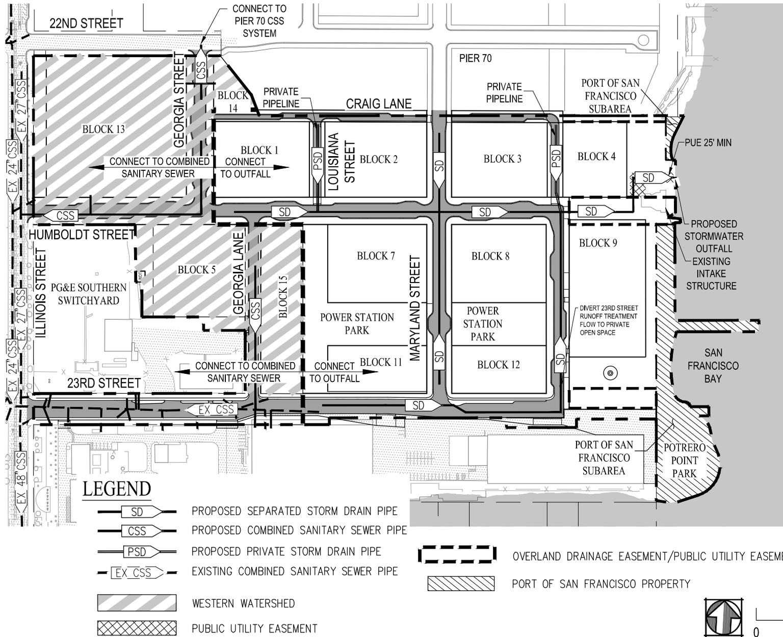
Figure 15.3 Proposed Storm Drain Systems
