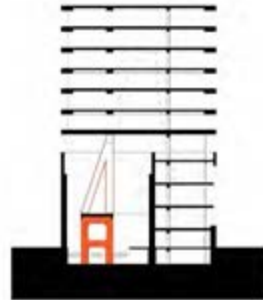
Integrating existing turbine foundation into structural system. Preserving/restoring existing brickwork & metalwork.
