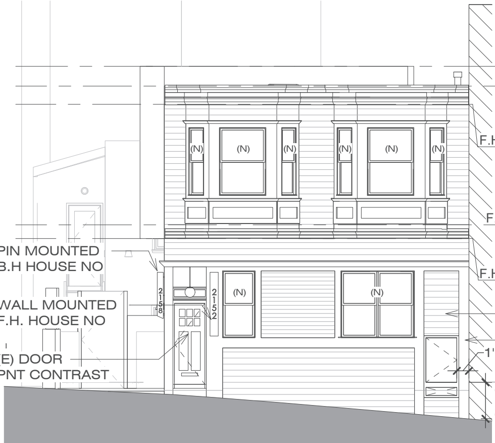
4 F.H. PROPOSED WEST ELEVATION 1/8" = 1'-0"
