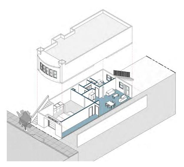
Most homes of this type have a narrow interior stair that connects the living space directly to the garage. With the ADU taking up much of the garage space this stair will likely need to be removed, and the opening in the floor above framed in, and finished to match the upstairs.
