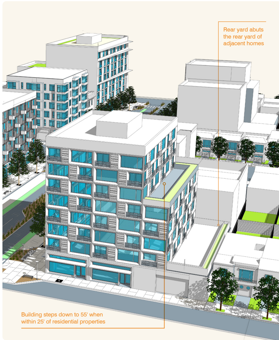
C.2.3 When rear yard of project abuts rear yard of a Residential Zoning District the building must step down to 55' when within 25' of lot depth.
