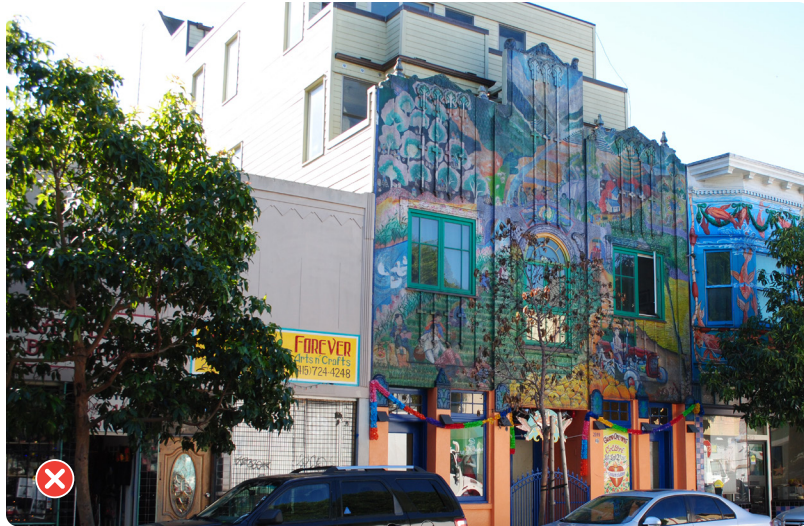
The rooftop addition at the right is not sufficiently set back, and overwhelms the historic building it is constructed on top of.
